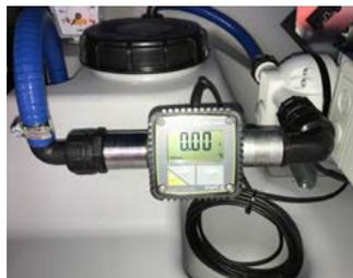
Meter FMT 3 with pulse output
