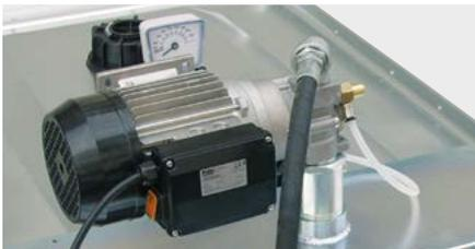
Pump 230 V (cannot be calibrated\*) with a delivery rate of 9 L/min and max. delivery pressure of 12 bar
