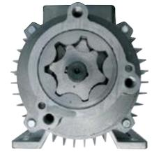
The pump principle: gear pump design
