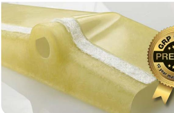
Due to the excellent material properties created by reinforcing the three-dimensionally meshed duroplastic material with glass fibres, GRP has been used for decades to make high-performance products that are expected to have a long service life in tough environments and at the same time ensure high levels of safety.
