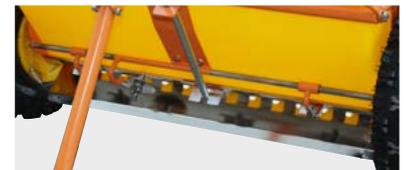
Rugged agitator shaft, axle divided in the middle
