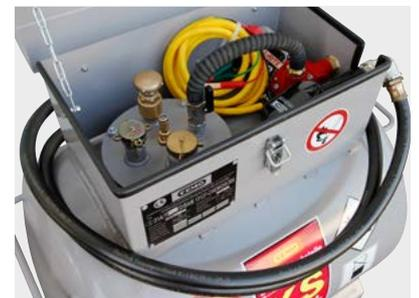
Pump cabinet (KS-MOBIL 200 L) with pump 12 V, 25 L/min, ATEX, 4 m discharge hose and automatic dispensing nozzle
