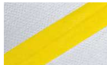
Stitched and taped seams. Optimum protection against penetration by liquid aerosols and solid particles.
